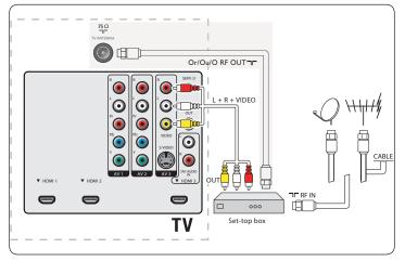
If your device has an S-VHS video jack: For improved picture quality, connect a S-Video cable with the S-Video input of AV3/side AV and connect the audio cables to the audio L and R input jacks of AV3/side AV.
